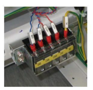
7. Note: the COM-SAN module may be also marked COM-PCS (as shown in the photos), however the functionalities of both interface modules are identical.
